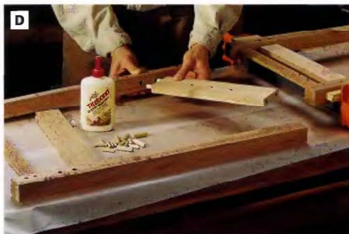
PHOTO D: Using dowel joints, glue and clamp up the legs and cross supports on a flat surface. Waxed paper protects your worksurface from glue spillage.
