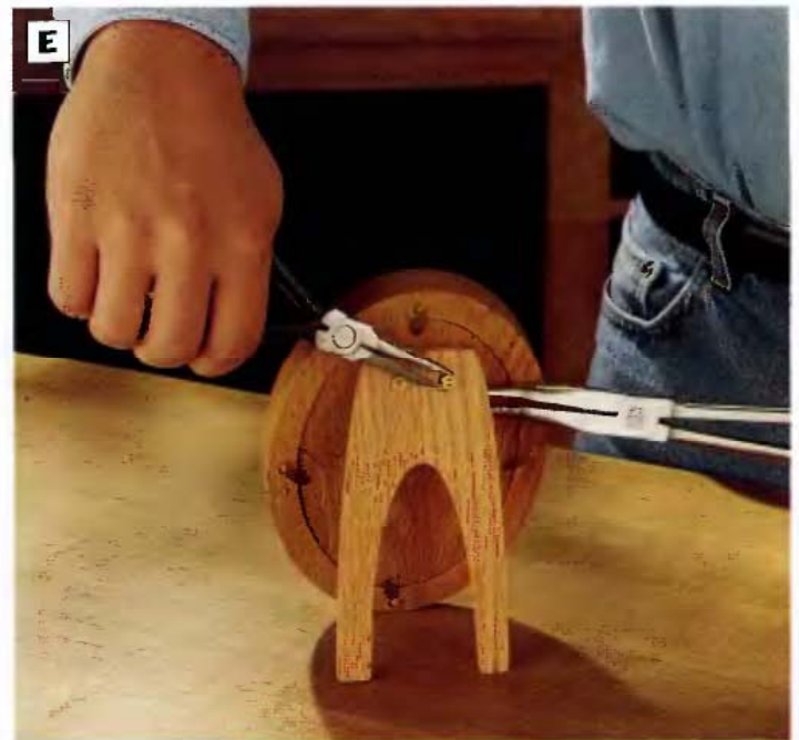
PHOTO E: After locating the hinge position, mount the hinge to the frame back with #4 × 1/4-in. brass flathead wood screws. Fasten the hinge to the stand with bolts and nuts. Arrange the bolts so you can thread the nuts on from the back of the stand. Tighten the nuts and bolts with a pair of needle-nose pliers.
