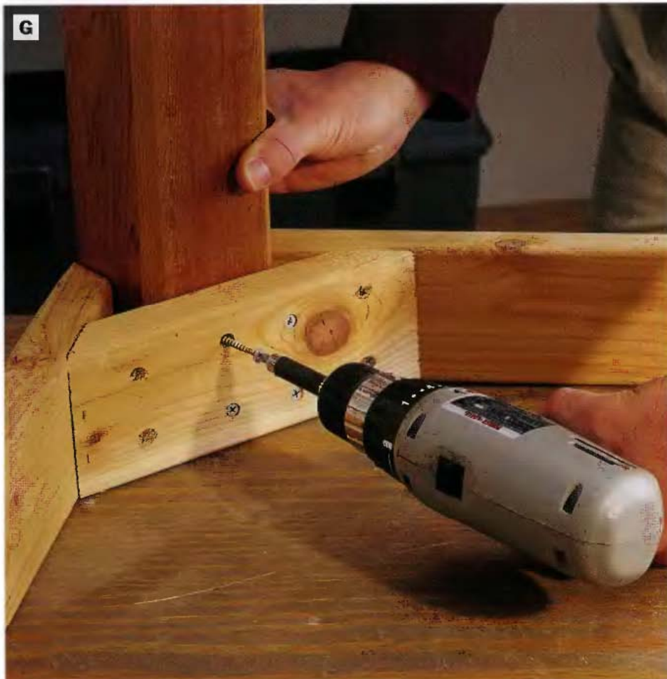
PHOTO G: Assemble the table legs, aprons and corner braces. Attach the parts by driving 2½-in. galvanized deck screws through countersunk pilot holes in the leg braces. Fasten the brace to each apron with a pair of screws driven in at an angle into the aprons, and use four screws for securing the leg. Be sure the legs are tight against the aprons and braces as you drive the screws.
