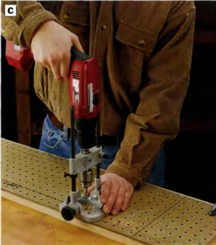
PHOTO C: Drill shelf pin holes in the sides of the upper cabinet, using pegboard as a template. Orient the guide the same way on facing sides to ensure that the holes are aligned.
