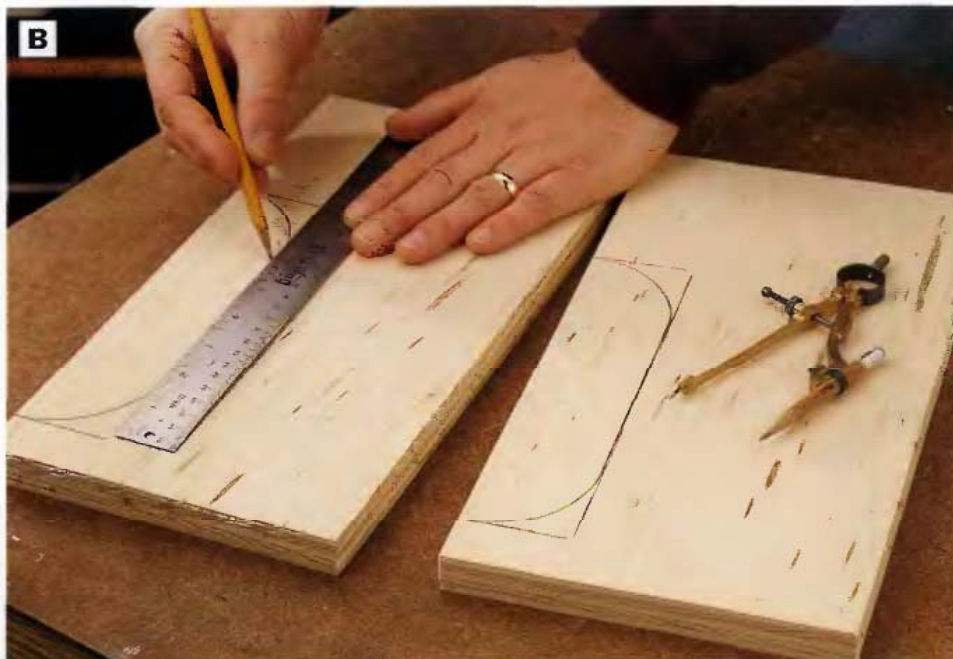
PHOTO B: Lay out the curves on the bench legs. Set your compass to draw a 2-in. radius to draw the arcs. Connect the layout lines with a straightedge.
