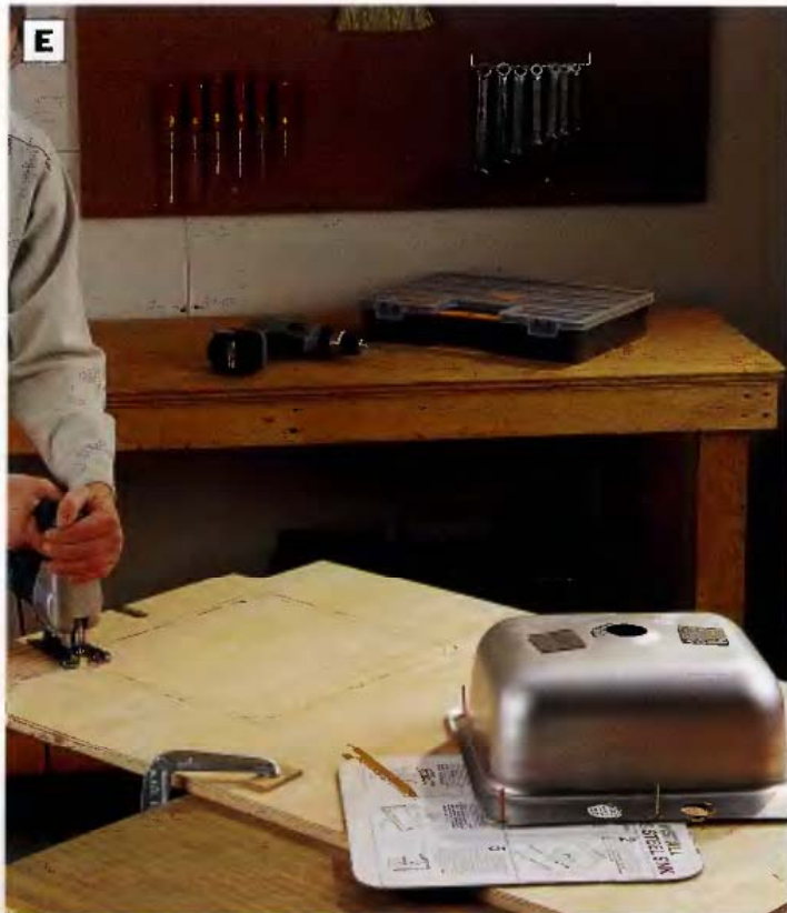
PHOTO E: Center the sink so it will hang over the storage area on the left side of the bench. Lay out the sink opening using the template provided by the manufacturer, and cut out the sink opening.
