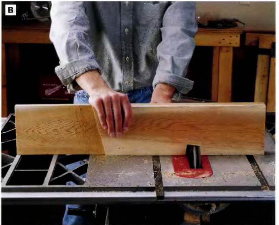
PHOTO B: Set the cutting angle of the dado-blade set to 7^\circ and cut 1-in.-deep notches for the seat supports into the bottom edges of the seat supports.
