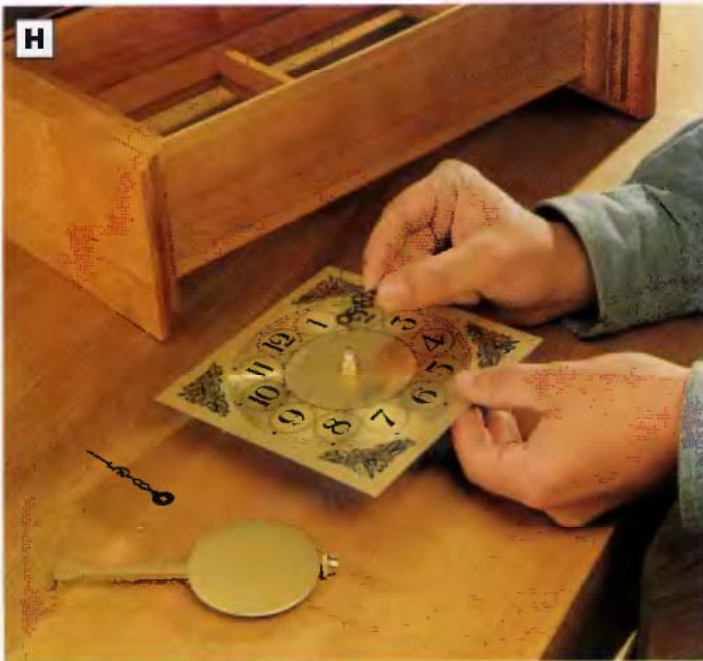
PHOTO H: Attach the quartz clock movement and hands to the clock face, according to the kitmaker's instructions.
