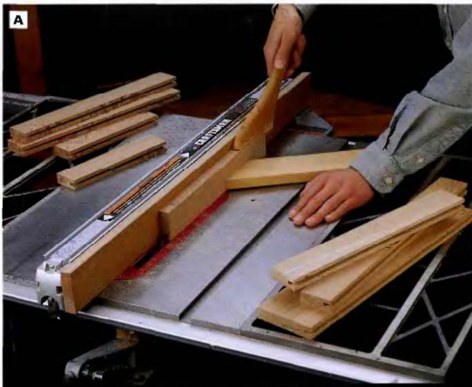
PHOTO A: Cut \frac{1}{4} \times \frac{1}{2} -in. grooves in the edges of the side and back rails and stiles. The grooves should be sized so the plywood panels fit into them snugly. Using a featherboard and pushstick, cut the grooves by making multiple passes with the table saw blade.
