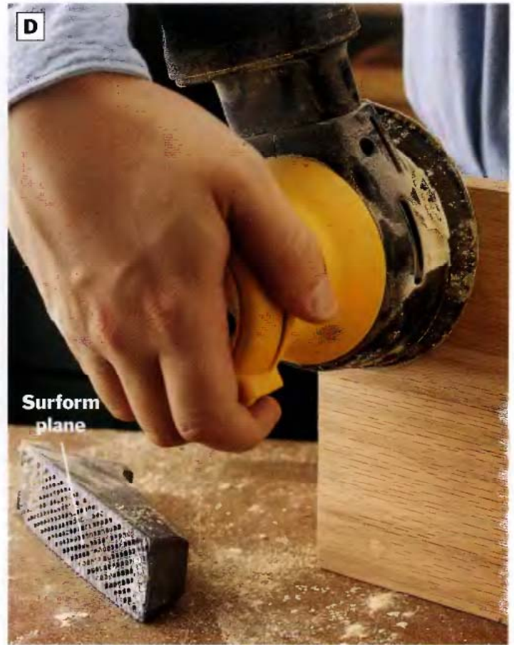
PHOTO D: Shave the plugs so they're nearly flush with the surrounding wood surface using a Surform plane or a wood rasp. Sand away the remaining waste with coarse sandpaper.
