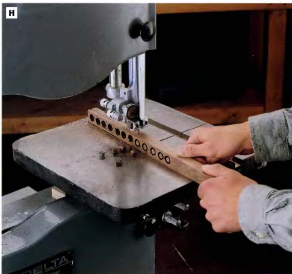
PHOTO H: Cut 16 to 20 plugs with the plug cutter, then resaw the walnut stock to about \frac{3}{8} -in. thick to release the plugs.
