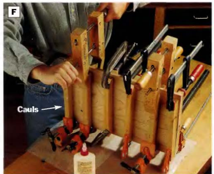
PHOTO F: Laminate two ¼-in. plywood sheets together to form the bottom panel. Clamp up the plywood on both sides with long wood cauls to press the sheets tightly together until the glue dries.
