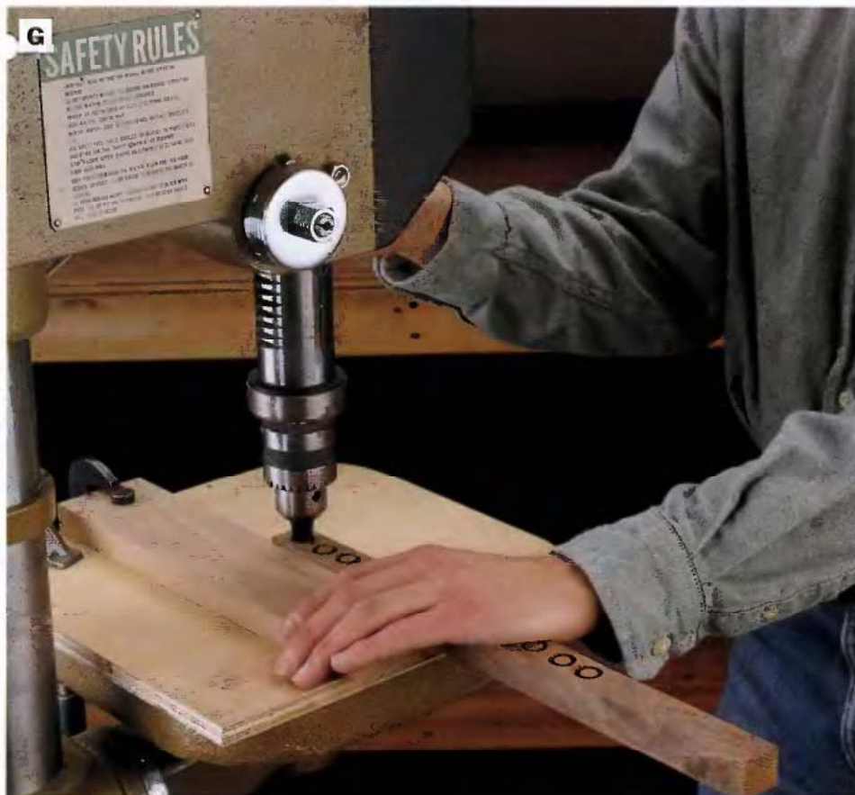
PHOTO G: Make walnut screw plugs on the drill press, using a \frac{3}{8} -in. tapered plug cutter. Clamp a scrap piece to the drill press table to create a surface that helps keep the walnut stock stationary while you cut the plugs.
