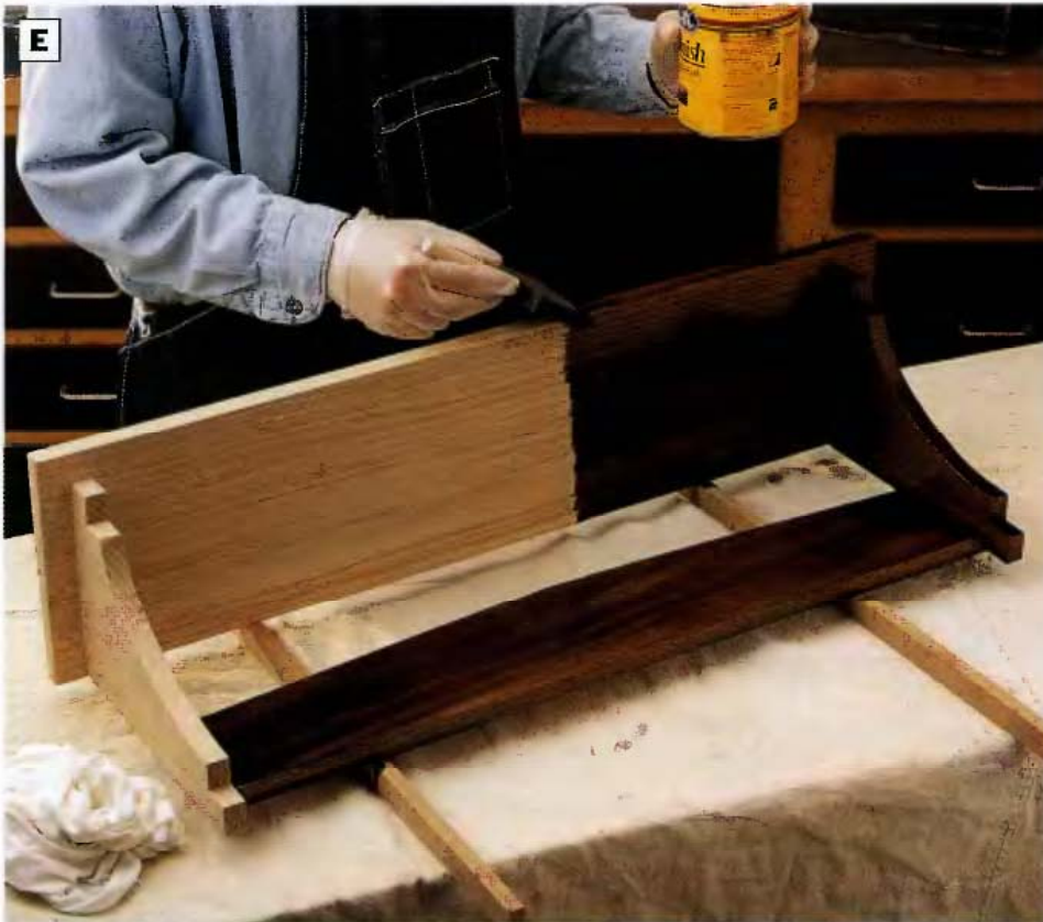
PHOTO E: Brush or wipe on a coat of wood stain with a foam brush or clean rag, then wipe off the excess stain before it dries. Wear disposable gloves to protect your hands. Topcoat the project with varnish.
