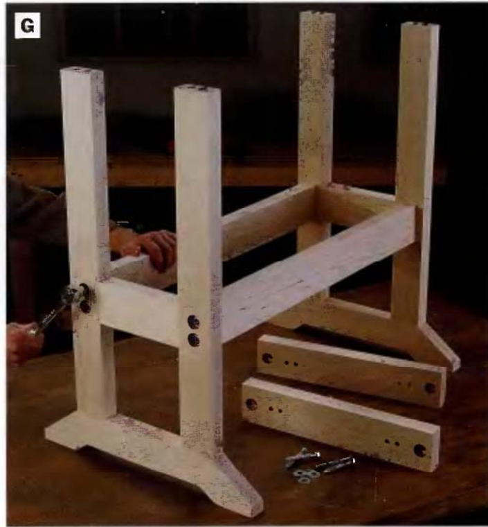
PHOTO G: After pilot holes are drilled, assemble the base with lag screws and washers driven with a socket wrench.
