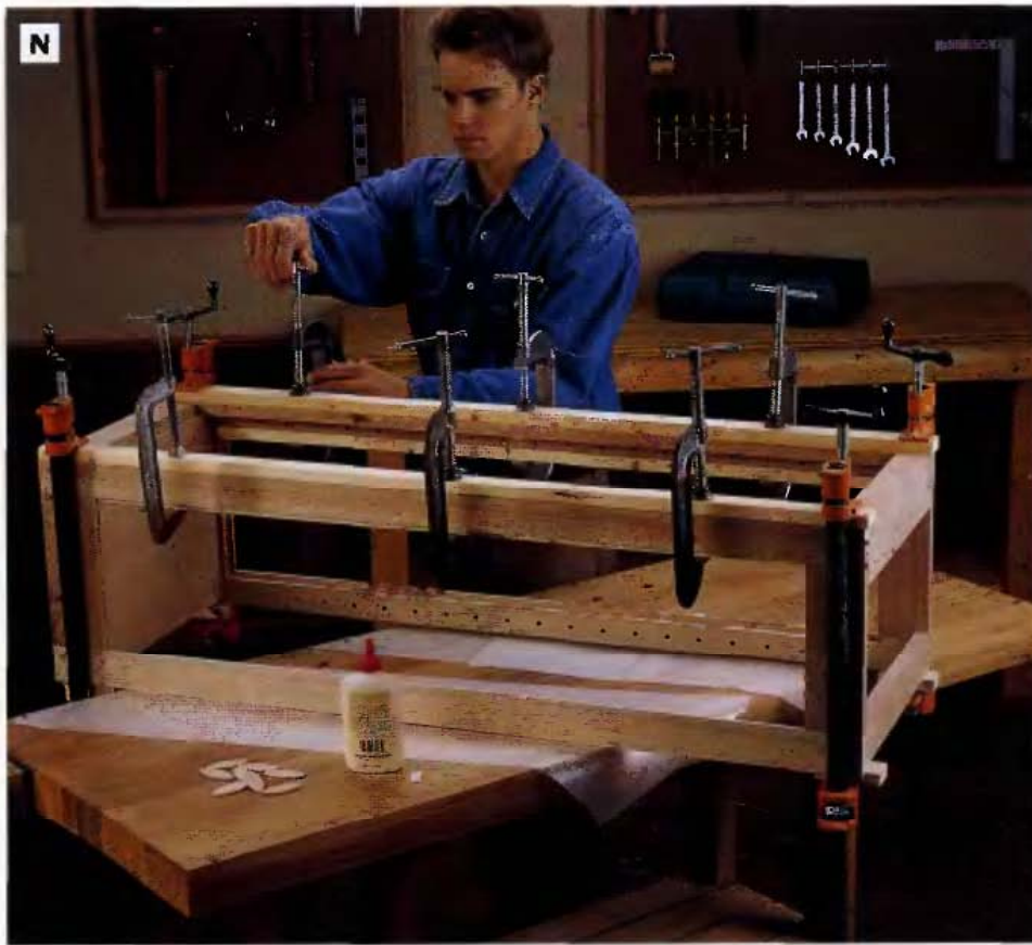
PHOTO N: Attach the face frame to the cabinet assembly with glue and biscuits, and clamp it up with a combination of C-clamps and pipe or bar clamps. Use full-length clamping cauls above and below the cabinet to distribute the clamping pressure evenly over the whole joint and to protect the cabinet parts from damage.
