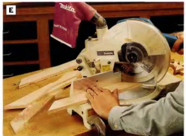
PHOTO E: Rip and crosscut the frame end and side pieces to size, then miter-cut the ends of the parts to 45°.
