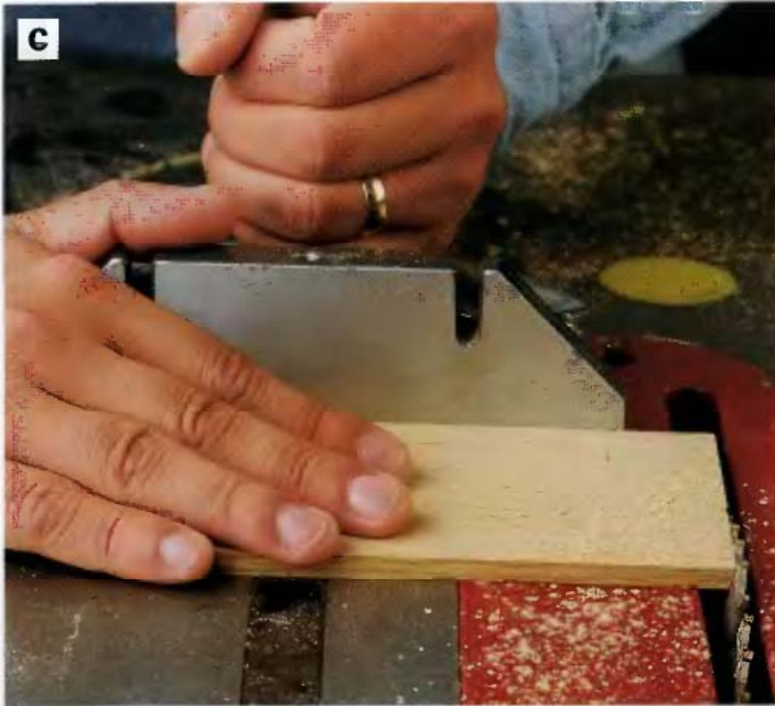
PHOTO C: Tilt the table saw blade to 13° and bevel-cut the top and bottom ends of the stand blank. Hold the workpiece against the miter gauge to make these cuts.
