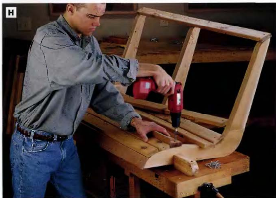
PHOTO H: Screw the slats to the back-and-seat support structures. Butt the first three slats together, then use a \frac{1}{4} -in.-thick spacer between the rest of the slats for consistent gaps. Keep the ends of the slats flush with the sides of the supports.
