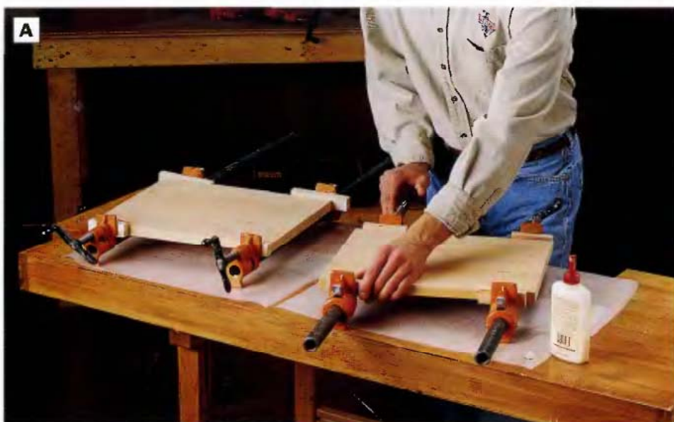
PHOTO A: Edge-glue panels for the sides and the bottom. As you tighten the clamps, the glue will cause the joints to slide out of alignment, so adjust them as well as you can to keep them lined up. Be sure to use clamping pads to protect the wood.
