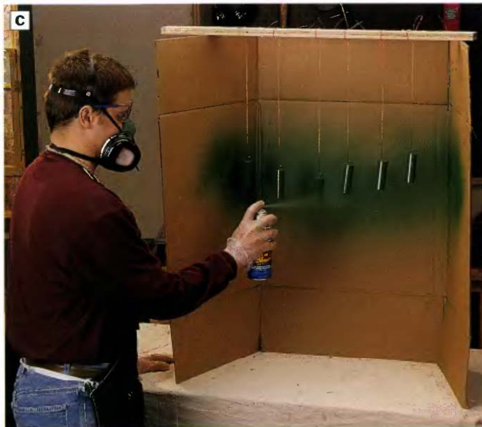
PHOTO C: Finish the blocks. We used primer and child-safe enamel spray paint. To make spraying easier, we hung the blocks with thumbtacks and string attached to a scrap of wood and suspended over a cardboard spraying shield. Wear a respirator if you use a spray finish.
