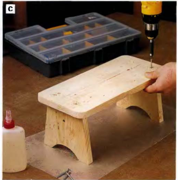
PHOTO C: Attach the top to the stretcher and legs with glue and screws. Lay out the stretcher and leg locations on the top first, for locating the screws.
