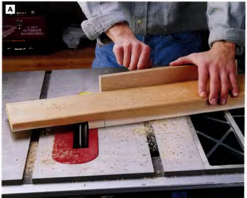
PHOTO A: Cut the half-laps in the seat supports and back supports with a dado-blade set, making multiple overlapping passes. The final pass on each board should be right along the marked cutting line. Set the miter gauge to 65^\circ . Making the half-lap joints prior to cutting the contours of the parts simplifies the layout of the contours.
