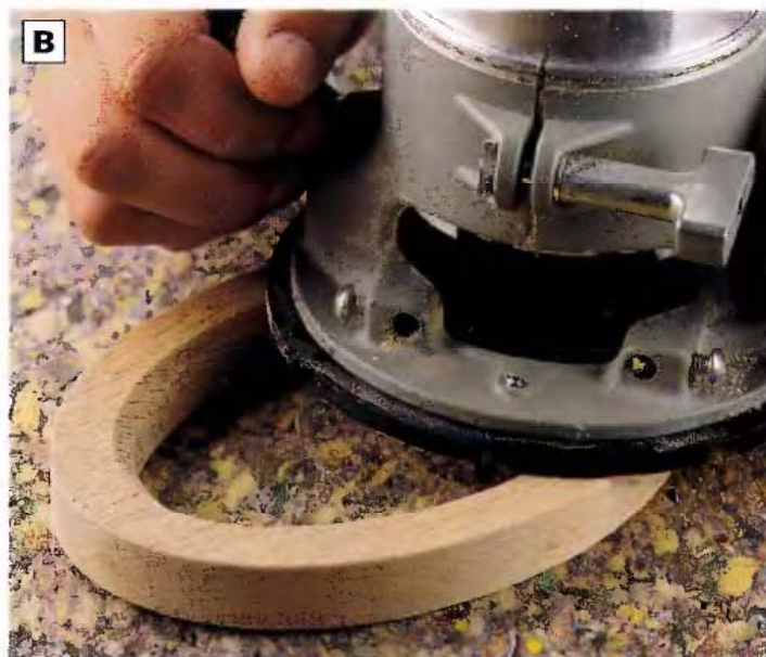
PHOTO B: Mill the 45° chamfer on the inside edge of the frame with the router held free-hand. Use a non-slip pad beneath the workpiece while you rout. Then turn the frame over, switch to a \frac{1}{4} -in. piloted rabbeting bit and rout the back rabbet around the inside edge.
