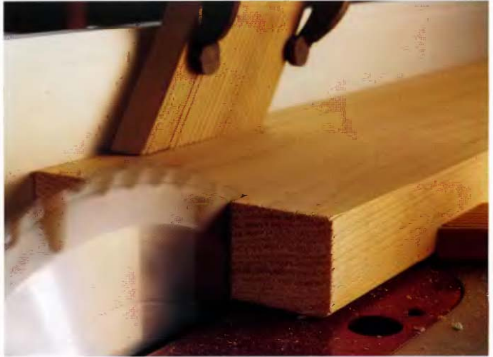
Ripping boards to width should be done after one edge has been squared (see previous section) so a flat even surface can ride against the saw fence or be used to register your straightedge for making rip cuts with hand-held tools.
