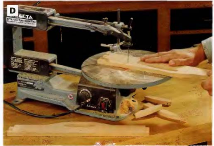
PHOTO D: Cut the curved handle profiles and cutouts on the scroll saw. You'll need to drill an access hole for the blade first, in order to start the handle cutout.
