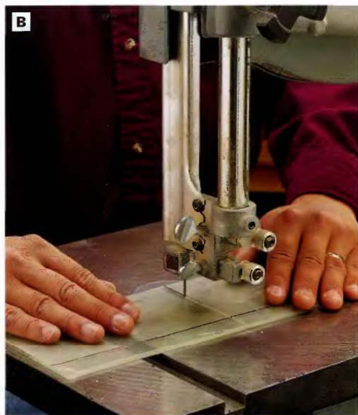
PHOTO B: Measure and cut the Plexiglas end panels on the band saw with a fine-toothed blade. Leave the protective film on the plastic as you machine it, to minimize scratching.
