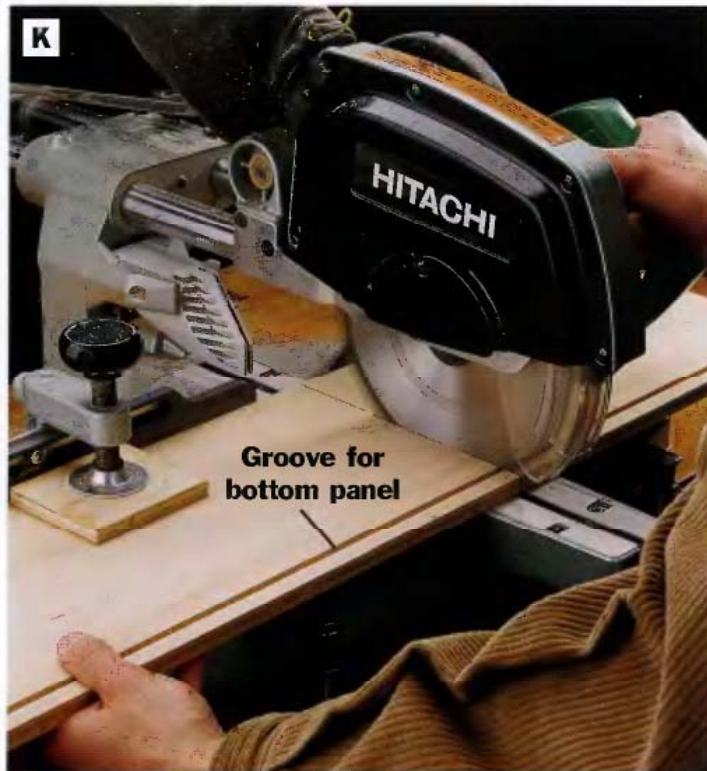
PHOTO K: The sides, front and back for each drawer can be cut from a single 8-ft.-long strip of \frac{1}{2} -in. plywood. By cutting the groove for the drawer bottom before cross-cutting the parts, you can ensure that the groove will line up on all four parts.
