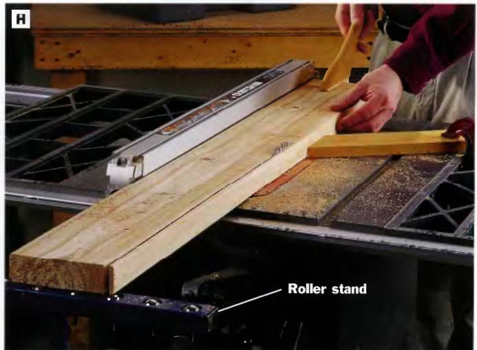
PHOTO H: Rip-cut 2 × 6 stock down to a width of 5\frac{1}{8} in. to form the tabletop slats. You could make these cuts with a circular saw and straightedge guide, but a better choice is to use the table saw and rip fence. Support workpieces with a roller stand as they leave the saw table.
