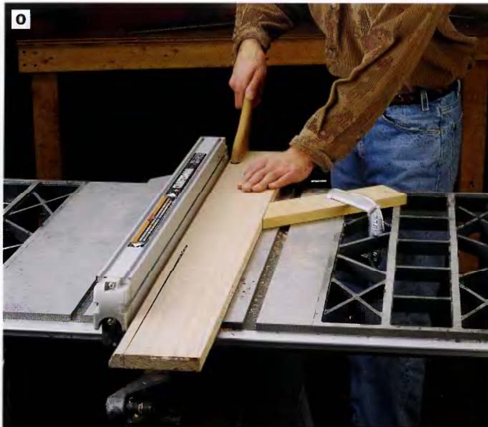
PHOTO O: After the molding profile has been routed into the edge of a wide, \frac{3}{4} -in.-thick oak board, rip-cut a \frac{3}{4} -in.-wide strip of the molding on the table saw. Repeat the process to make up as much molding as you'll need (about 13 lineal feet for the project as shown). This process is easier and safer than ripping the molding to width first and trying to feed narrow strips across a large cutter on the router table.
