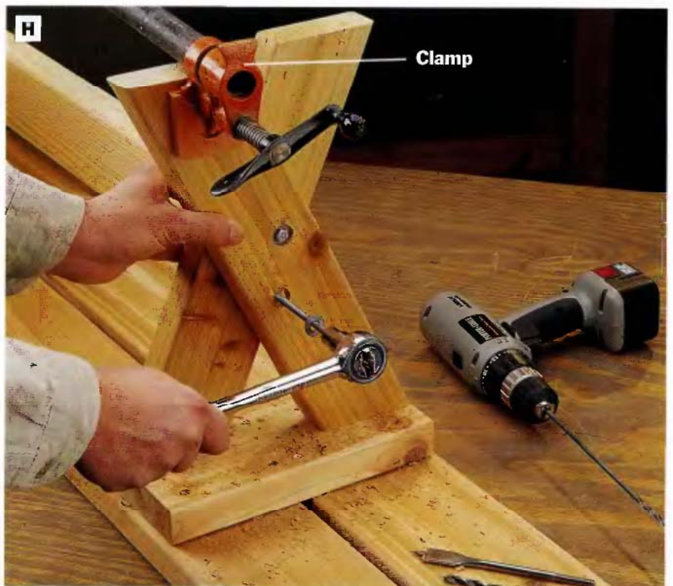
PHOTO H: Cut the bench braces to length and clamp them in position 5 1/2 in. from the bottoms of the legs on each bench. Drill 3/4-in.-dia. counterbores in the outermost legs to recess two lag bolt heads, then drill pilot holes through the counterbored holes to install the lag bolts. Slip a washer onto each lag bolt before you screw it through the legs and into the bench braces.
