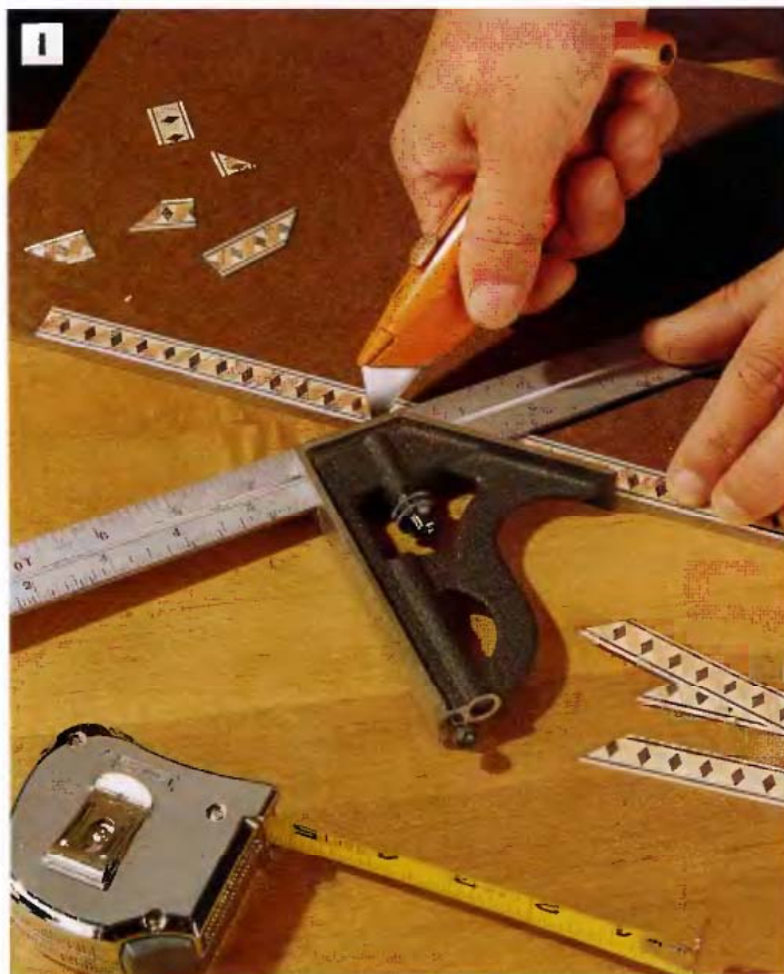
PHOTO I: Miter-cut the corners of the decorative inlay strips using the 45° fence on a combination square and a sharp utility knife. Hold the knife as square to the inlay as you can when making the cuts, so the mitered joints will meet flush.
