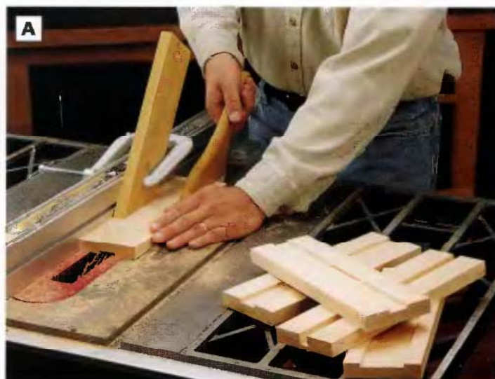
PHOTO A: Cut the knife slots into one face of the strips using a dado blade on the table saw (as shown), or on a router table with a straight bit and fence.
