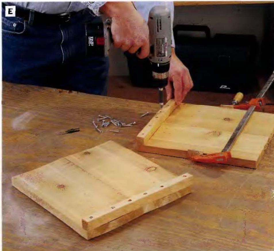
PHOTO E: Clamp pairs of 6-in.-wide boards for the end panels and fasten each panel together with a cleat. Use 1½-in. galvanized screws to join the parts. These two cleats are permanent parts of the planter.
