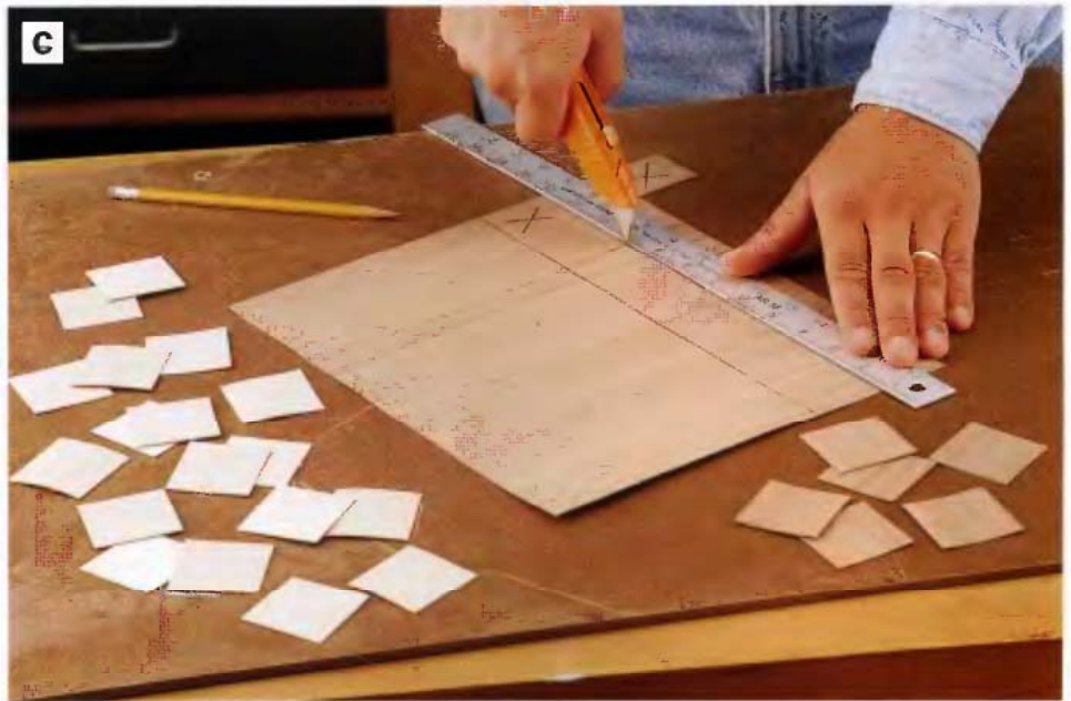
PHOTO C: Lay out and cut the chessboard squares from walnut and maple self-stick veneer. Make 32 of each, using a straightedge and utility knife to cut them out. Hold the blade vertically as you cut so that the edges will be square and fit tightly together.
