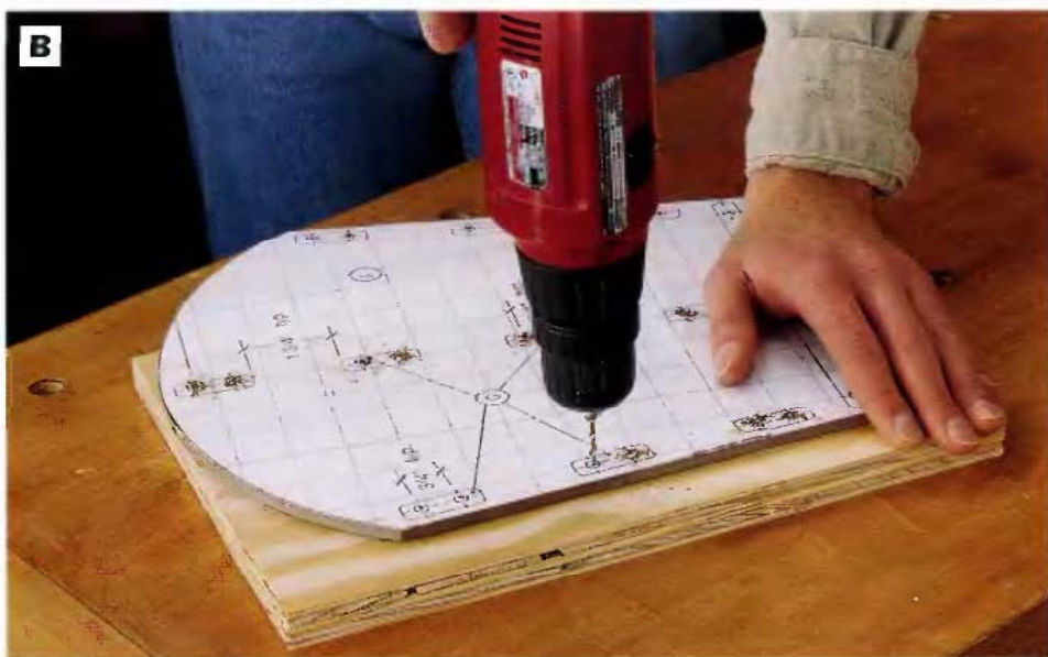
PHOTO B: Drill small locator holes through the side template, at the centerpoints shown for each dowel location. Use scrap plywood underneath to prevent drill bit tear-out.
