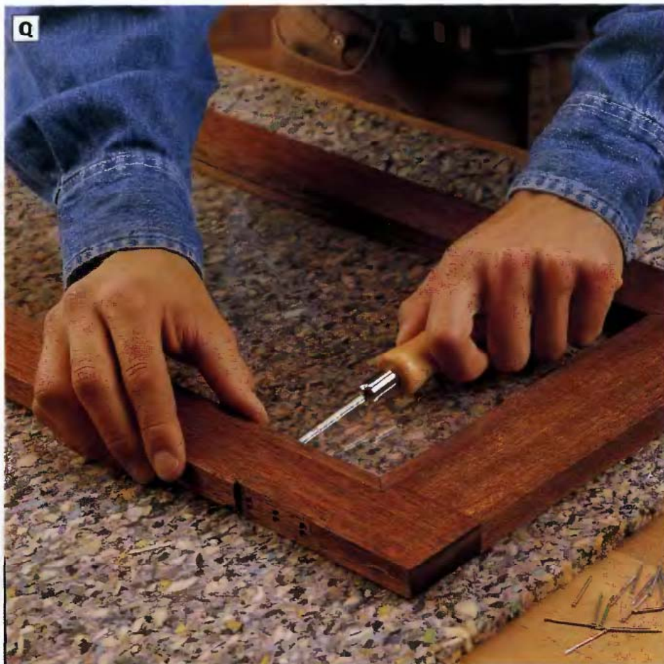
PHOTO Q: Set the glass into the recess in the door, and nail the mitered retainer strips in place. We drilled pilot holes in the strips first to make driving the nails easier. A brad driver (shown here) allows you to push the nails into place rather than swing a hammer close to the glass.
