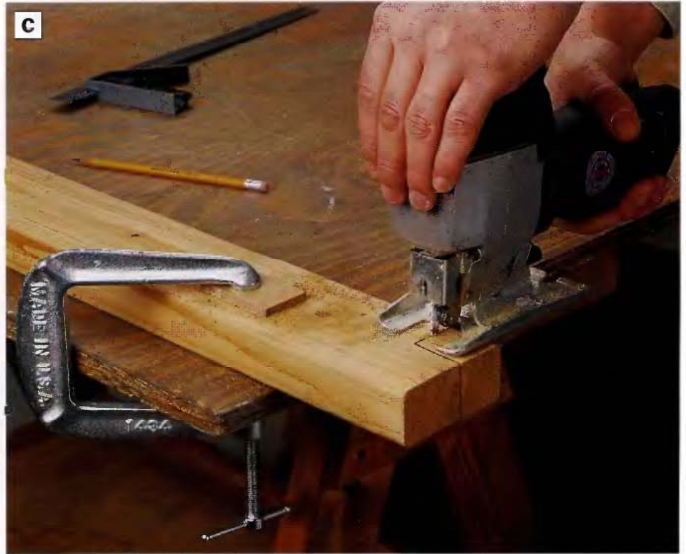
PHOTO C: Notch the top front corner of the center front leg so it will fit around the top front stretcher. Then combine this leg with the rear support, drawer stretcher, drawer slide and lower stretcher to form the middle support assembly.
