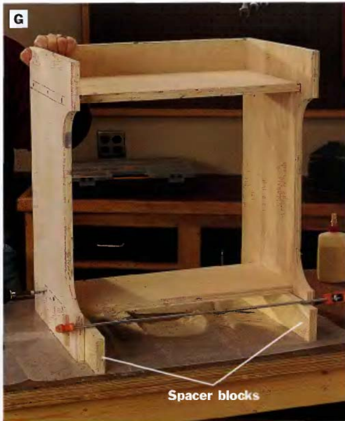
PHOTO G: install the footrest with glue and screws. Insert a couple of 3¼-in.-wide spacer blocks beneath the footrest to hold it in position temporarily while you screw it in place.
