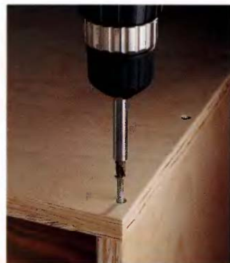
WOOD SCREWS are popular fasteners for reinforcing butt joints. They should be driven into counterbored or countersunk pilot holes.
