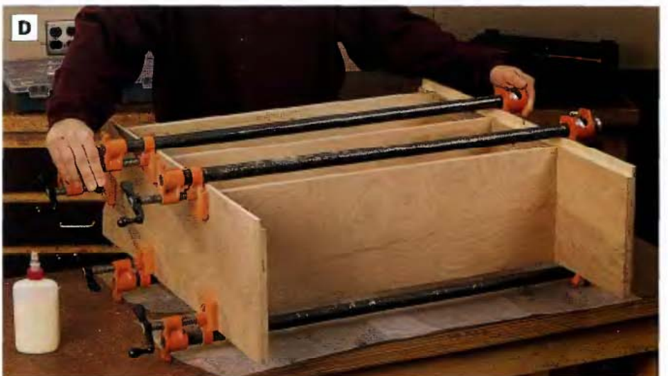
PHOTO D: Glue and clamp the shelves into their dadoes in the bookcase sides. Keep the shelves flush with the front edges of the sides so they don't obstruct the back rabbets.
