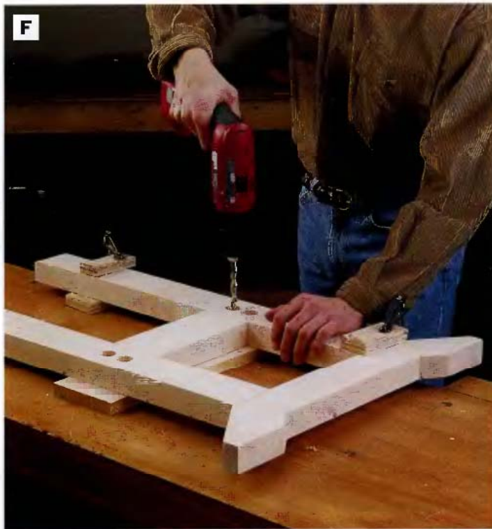
PHOTO F: Drill counterbore holes for the lag screw heads and washers, and drill clearance holes and pilot holes for the shanks of the screws.
