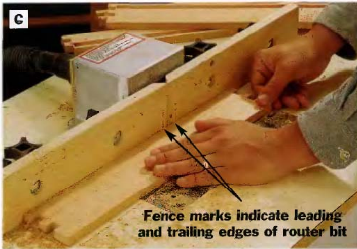
PHOTO C: Cut the bottom panel grooves in the tray sides and ends on the router table. When cutting these stopped dados on the tray sides and ends, mark the leading and trailing edges of the bit on the router fence so you know where to start and stop the cuts.
