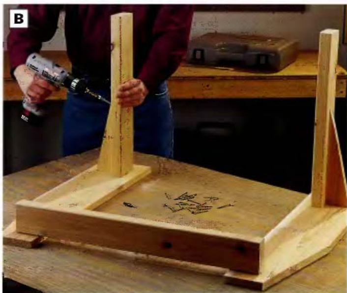
PHOTO B: Attach the back support, front legs and arm braces to the arm workpieces with 2-in. galvanized screws.
