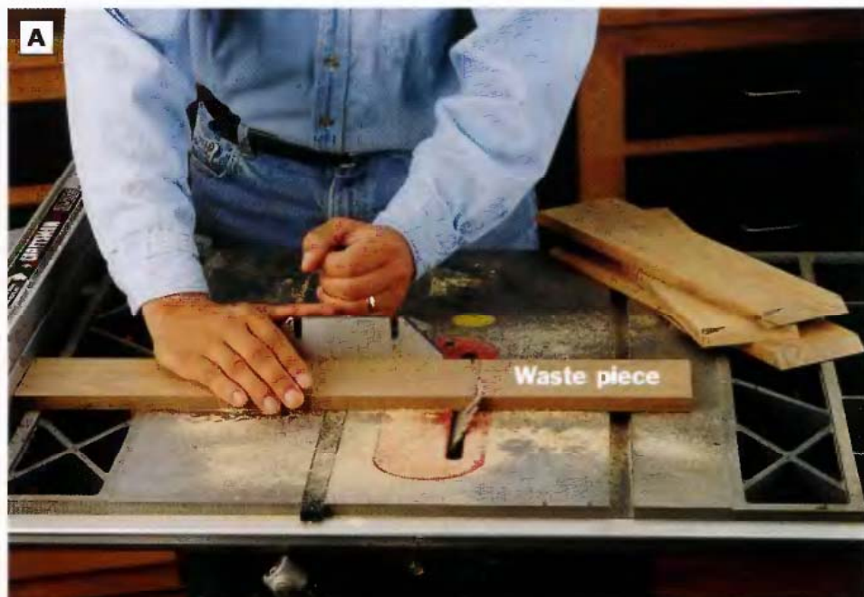
PHOTO A: Crosscut the front, back and side pieces to length on the table saw with the blade tilted to 45^\circ . Since all four parts are the same length, you can use the saw fence as an index to establish the length of the parts, like we show here. CAUTION: If you use this method, the blade must tilt away from the fence, and the waste piece must fall away on the side of the blade opposite the fence. Otherwise, the waste piece or the workpiece could become trapped between the blade and the fence and result in kickback.
