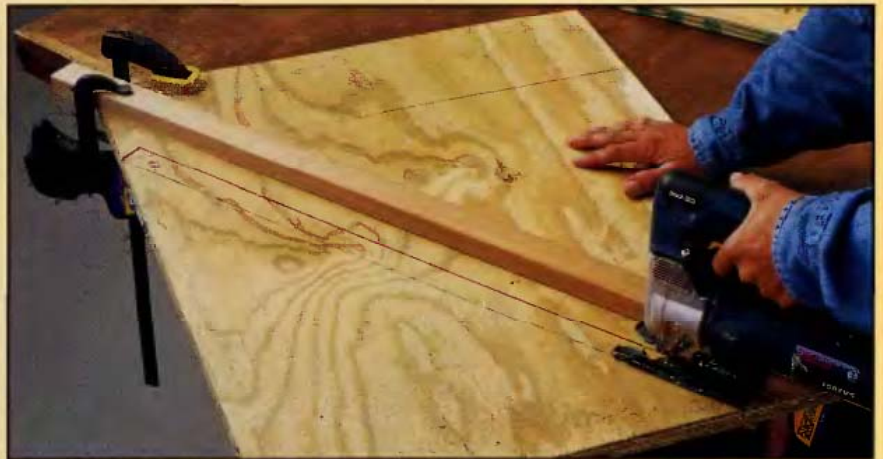
RIP-CUTTING WITH A JIG SAW: One advantage to using a jig saw to make rip cuts is that it's easy to set up a straightedge and make a cut that's not parallel to the edge of the board. Be sure the guide is set to allow for the offset between the saw foot and blade.
