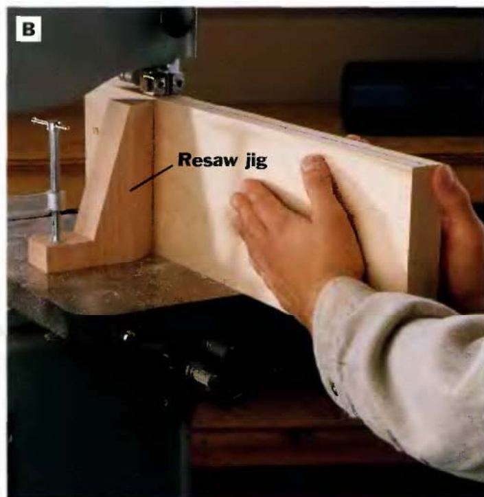
PHOTO B: Resaw the maple stock in half for the sides and ends of the box, using a marked centerline as a guide for the blade. A shop-made resaw jig clamped to the saw table will help square the board to the table and keep the blade tracking along the cutting line.
