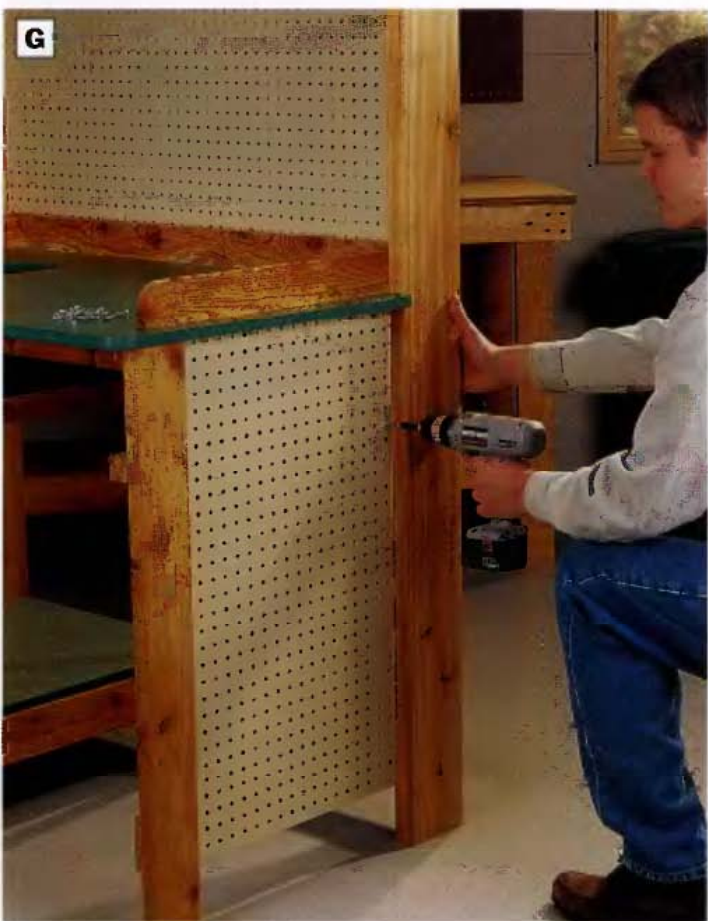
PHOTO G: Fasten the perforboard side and back panels to the bench framework with 1½-in. galvanized deck screws. Be careful not to overdrive the screws when installing the perforboard.
